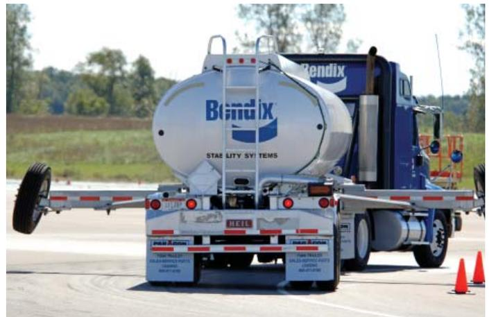
With the Bendix ABS-6 with ESP® activated, the vehicle repeats the course navigating the same maneuver safely.
