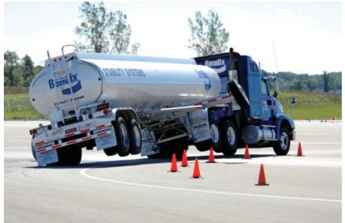
Above image shows a vehicle on a test track in a potential rollover scenario - note outrigger position.
