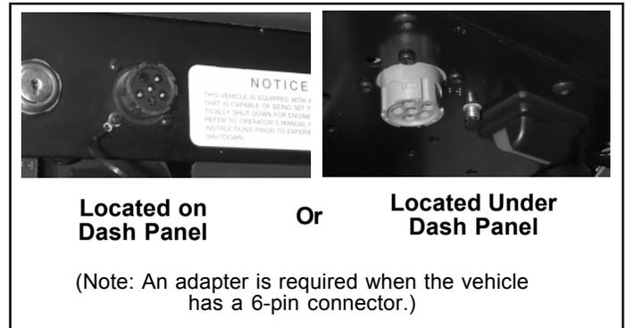
FIGURE 2 - TYPICAL VEHICLE DIAGNOSTIC CONNECTOR LOCATIONS (J1708/J1587, J1939)
