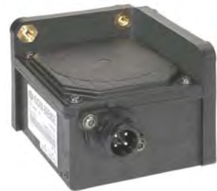
Bendix® YAS-60™ Yaw/Lateral Acceleration Sensor Package
