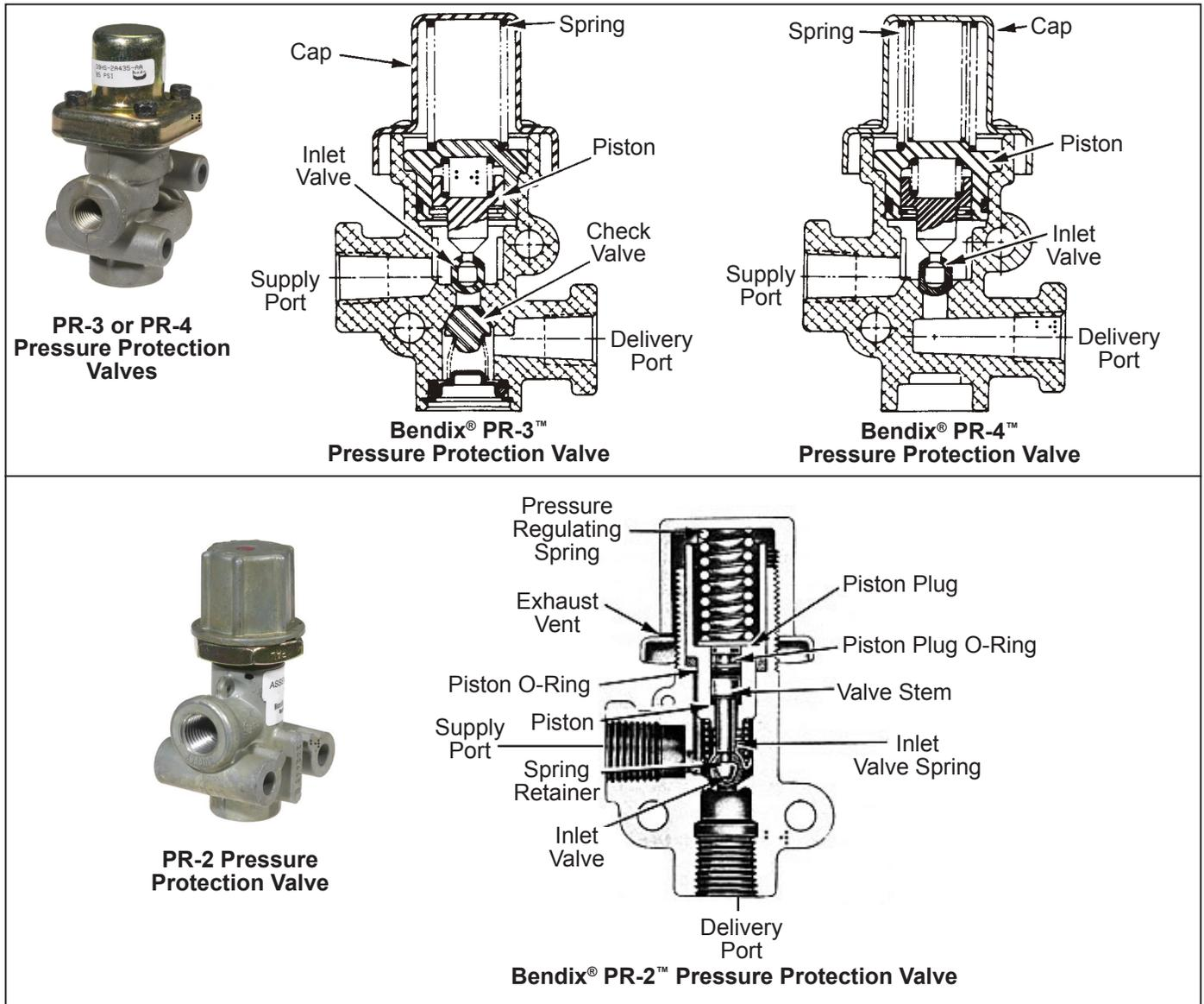
Figure 1 – Bendix® PR-2™, PR-3™ & PR-4™ Pressure Protection Valves
