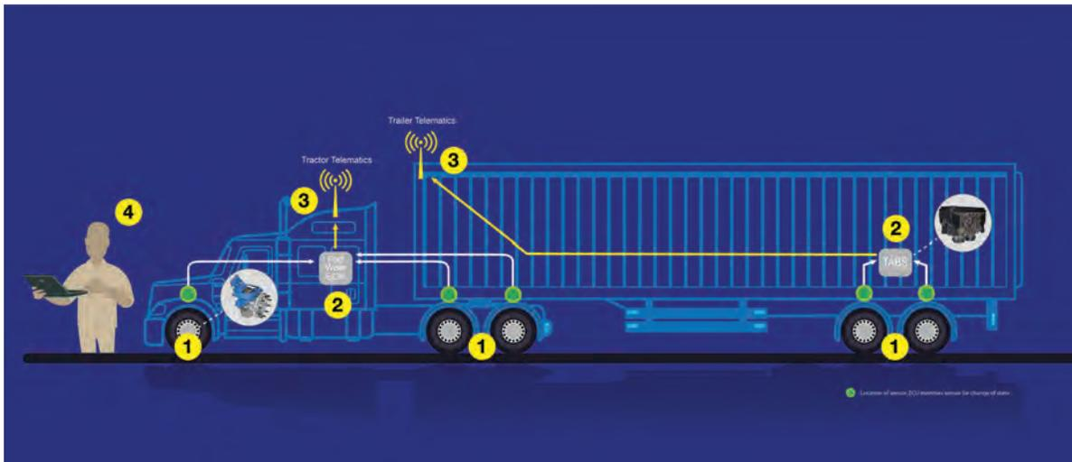
1. The sensor detects that the pad is nearing replacement condition; time to schedule maintenance
