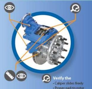
Proper pad-to-rotor running clearances
