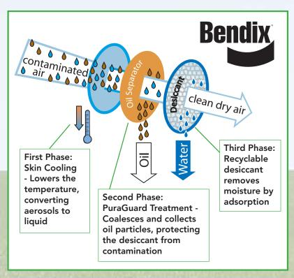
Bendix integrates proven PuraGuard® oil coalescing technology into the air dryer cartridge.
