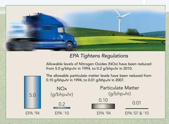
Manufacturers responded to EPA '07 and '10 with major technical advances to their vehicle systems. These advances – including Advanced Exhaust Gas Recirculation (EGR), Selective Catalytic Reduction (SCR), and the Diesel Particulate Filter (DPF) – have added a total of \$10,000 to \$15,000 to the cost of each commercial vehicle. As costs rise, so does the pressure to protect your investment.
