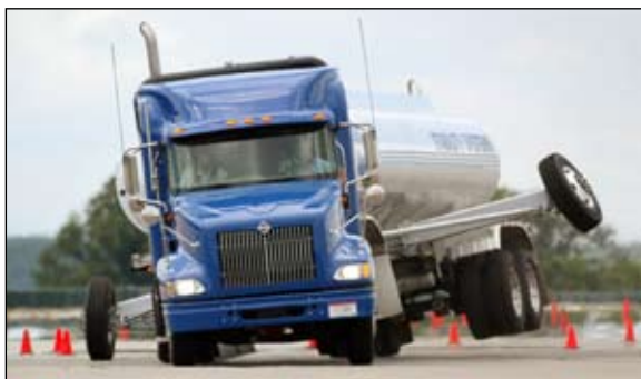
During demo and testing of stability systems, trailers and straight trucks are outfitted with outriggers to enable full rollover simulation.
