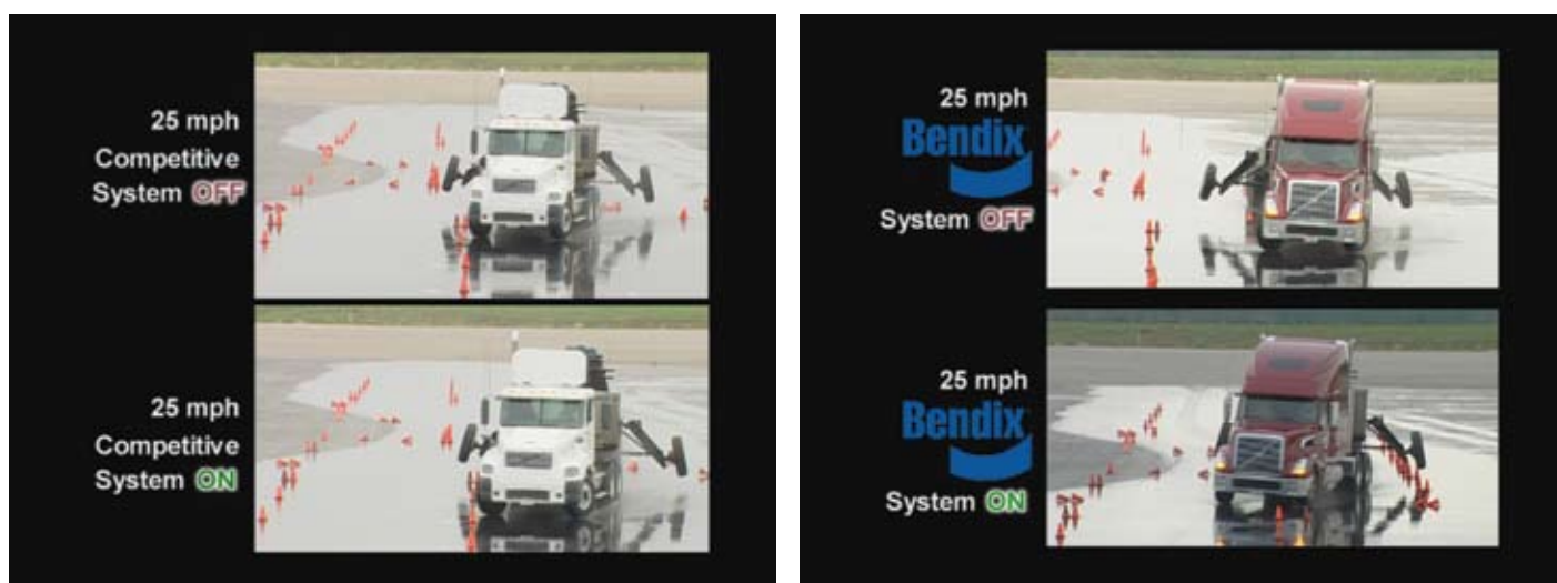
The photos above illustrate the performance of full-stability (the red vehicle) versus roll-only (the white vehicle) systems on a slick surface avoidance maneuver at identical speeds. The white, roll-only, truck is not able to stay in the lane, while with the full-stability system engaged, the red truck maintains position throughout the maneuver.
