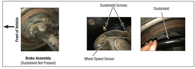
3. Visually inspect the brake spiders for the presence of cracks as shown below.
